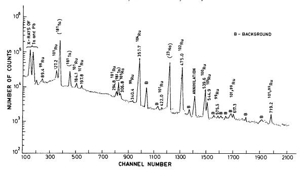
Fig. 1. A typical gamma-ray spectrum from Coulomb excitation of Ru isotopes at 3.0 MeV incident proton energy.
