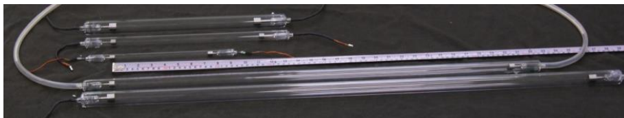
Xenon Flashlamps of arc length 200 to 900 mm developed in India with M/s Litex Ltd., Pune
