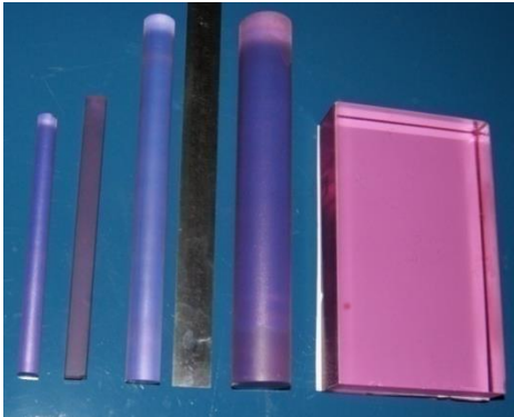
Nd:phosphate glass rods/discs from CGCRI
